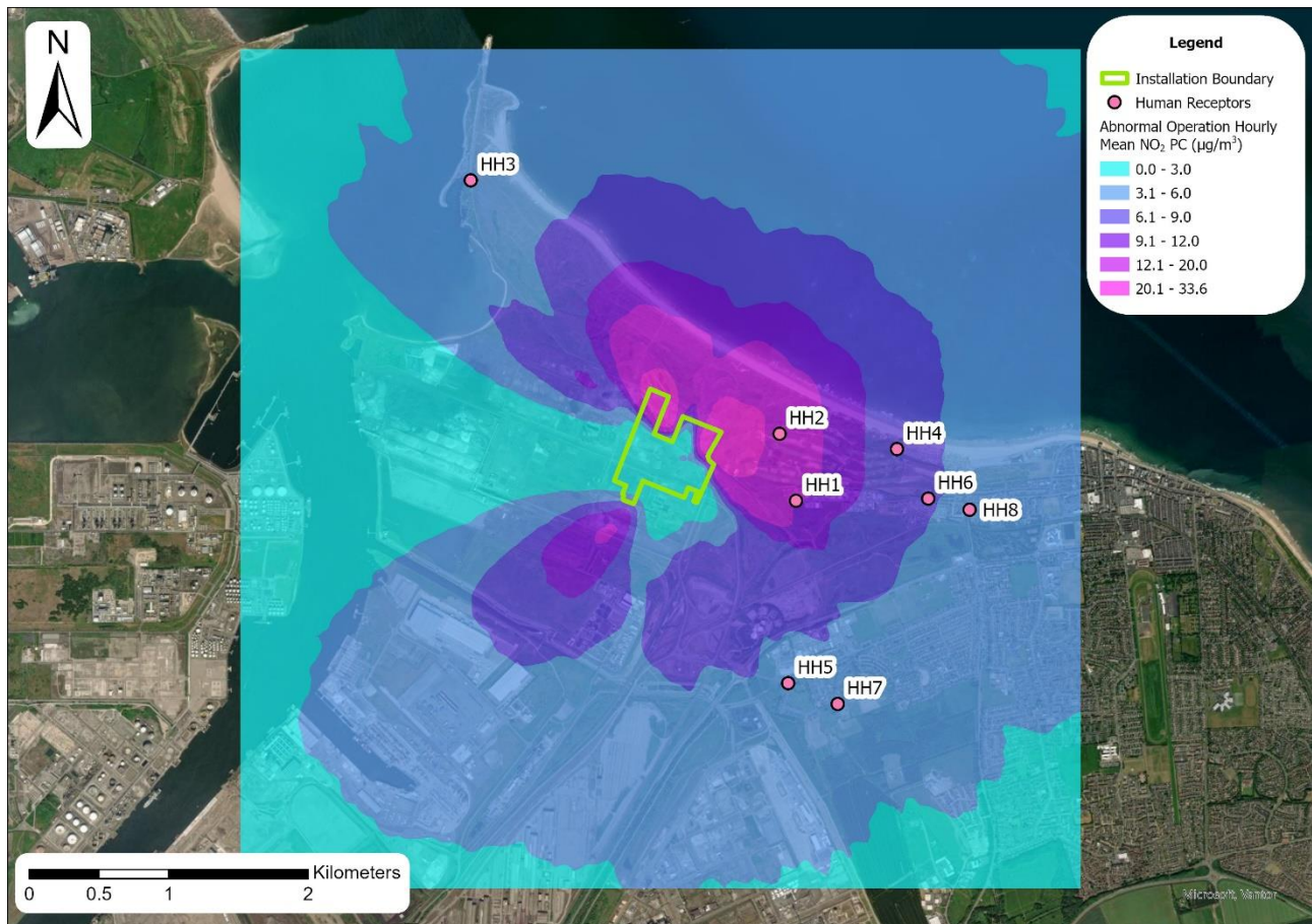
Figure 11: Scenario 2 – Abnormal Operation Isopleths of the Predicted Hourly Mean NO 2 PCs (µg/m 3 )
